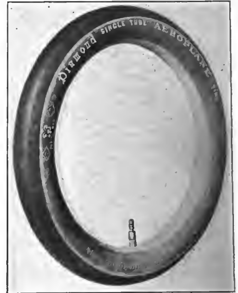
Leather-tread tire for aeroplanes
